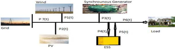
Fig. 1. Power system configuration of micro grid
